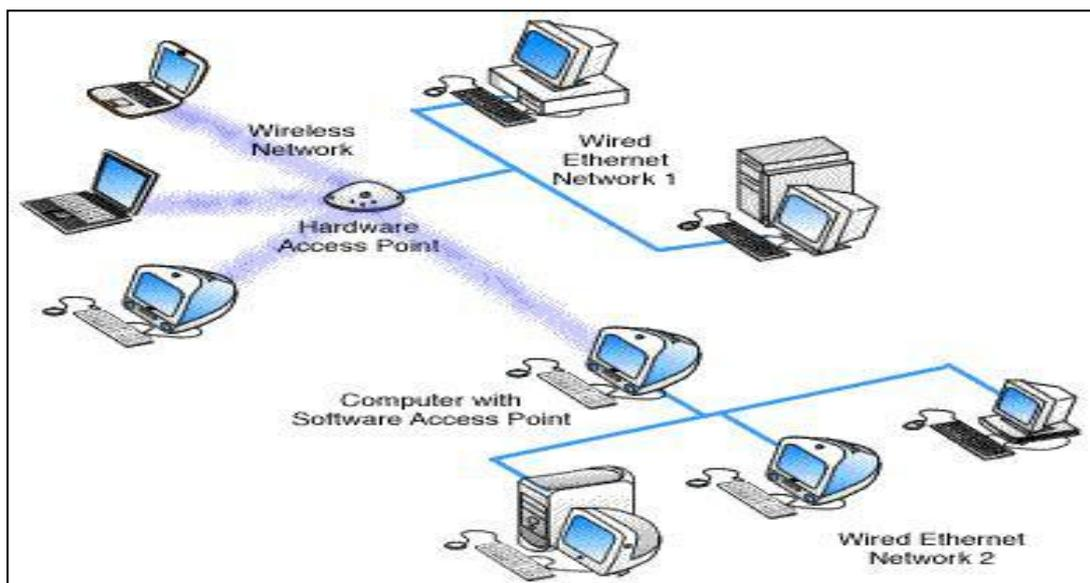
APs may also provide a “bridging” function. Bridging connects two or more networks together and allows them to communicate—to exchange network traffic. Bridging involves either a point-to-point or a multipoint configuration. In a point-to-point architecture, two LANs are connected to each other via the LANs’ respective APs. In multipoint bridging, one subnet on a LAN is connected to several other subnets on another LAN via each subnet AP.
