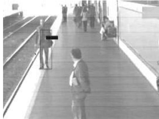
**Fig.1 Pedestrian automatically identified as too close to platform edge (marked by rectangle and bar)**
