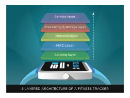
• Sensing layer: This layer has sensors embedded in the device; these sensors collect data like number of footsteps, heart rate, body temperature, etc. The data collected by sensors are sent to servers using Wide Area Network such as GSM, GPRS, and LTE.
