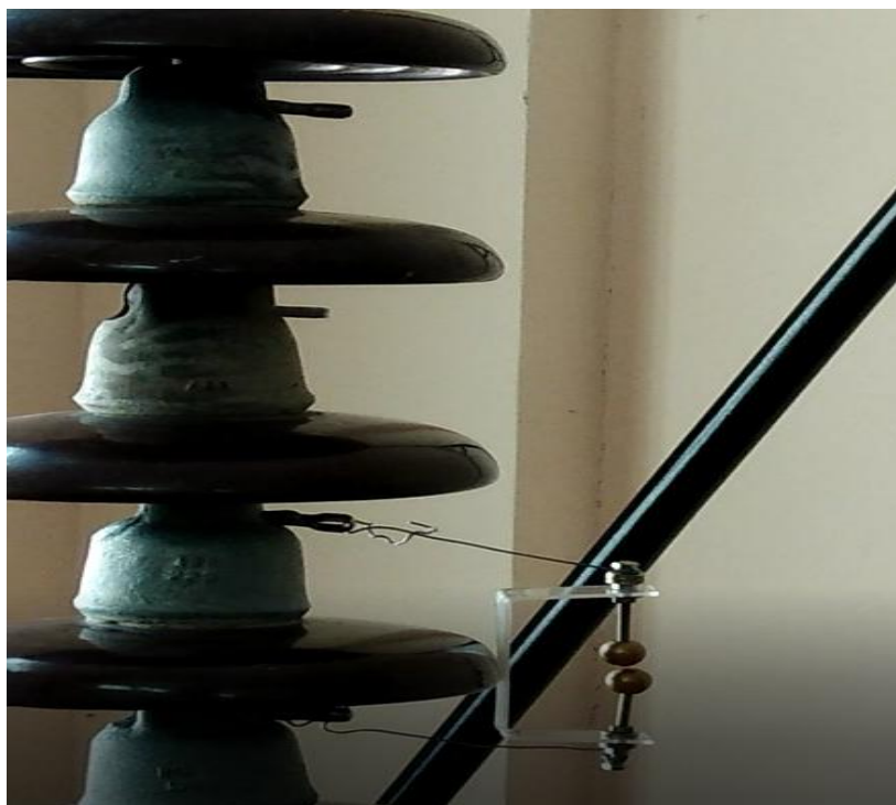
Fig.2 Arrangement of voltage distribution without guard rings
