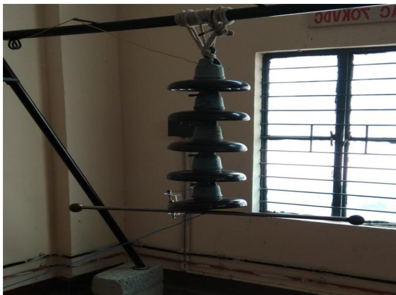
Fig.4The arrangement of voltage distribution with guard rings and the theoretical values is calculated as below
