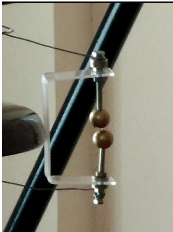
Fig.3 Sphere gap arrangement with the appearance of spark between the spheres without guard ring
