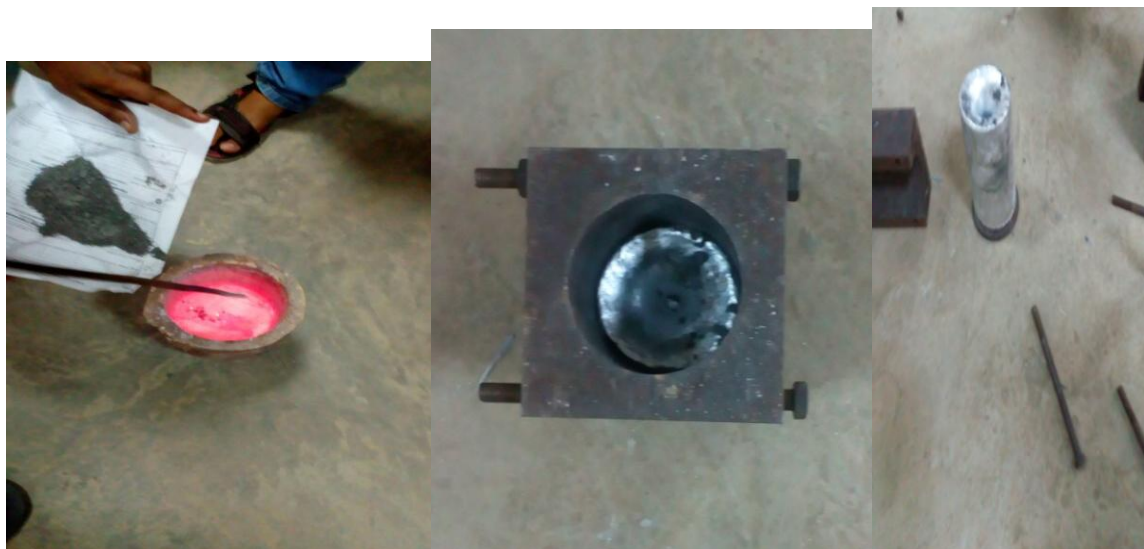
Fig 3: Preparation of INGOTS
