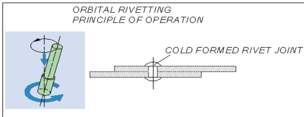
**Fig.1:- Orbital riveting principle of operation**
