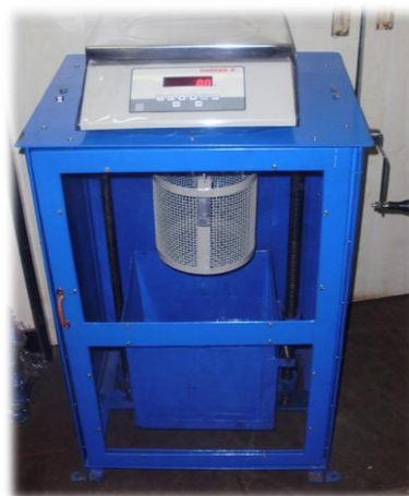
FIGURE 5. Specific Gravity Test With Help Of Mesh Bucket
