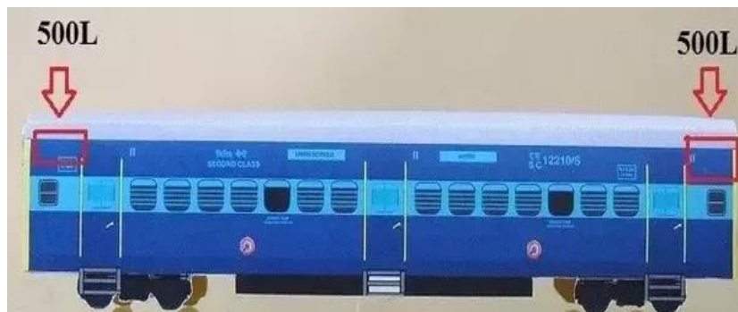
Fig e Water storage
