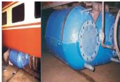
Fig d Water Tank
