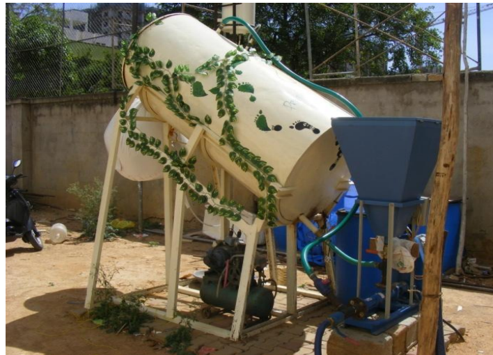
Fig 3- Picture of Biogas plant
