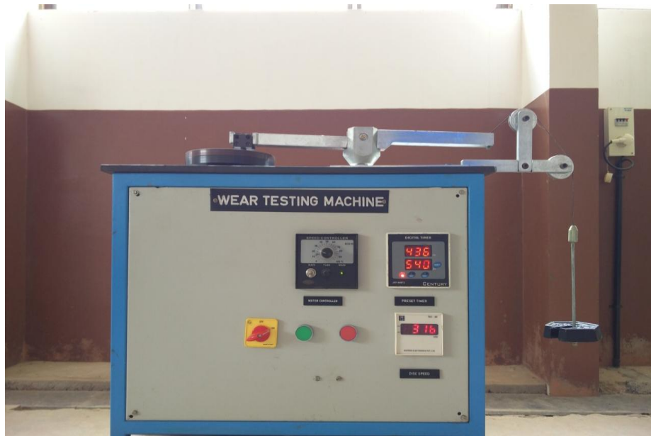
Fig 1: Pinon Disc testing rig
