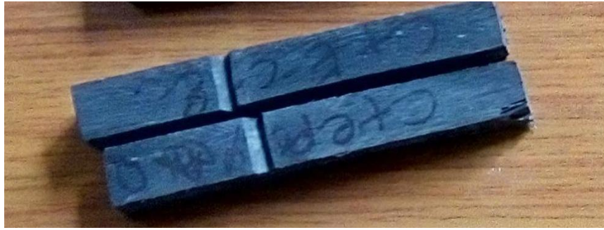
Fig 5: Impact Specimen of Carbon/Epoxy
