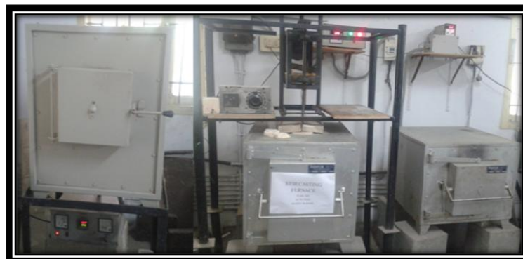
Fig 2: Stir Casting Set-up used for fabrication of Composite Plates (Al 7075/WC)
