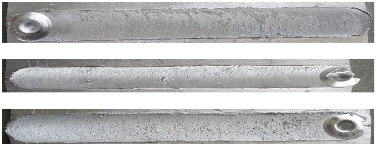
Fig 4: Photographs and Visual inspection of welds 1120 rpm and feed rates of 50, mm/min 2° tool tilt angle and tool pin profile
