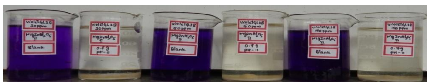
Photo 3: Effect of initial dye concentration on the photocatalytic degradation of Violet GL2B [ MgZnAl_2O_5 (acetamide) g/pH=0.7/11 and Violet GL2B = (30, 50 and 70) ppm]
