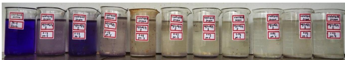
Photo 1: Effect of catalyst concentration on Violet GL2B at 120 minutes [Violet GL2B =30 ppm, pH=7, MgZnAl 2 O 5 (acetamide)]
