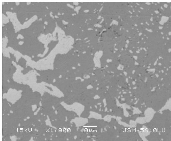
**Fig.(c): SEM micrograph for 19.54 At. % Bi and 80.46 At.% Sn.**
