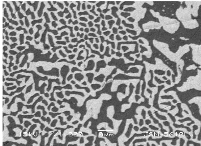
Fig.(f): SEM micrograph for 37.99 At. % Bi and 62.01 At.% Sn.
