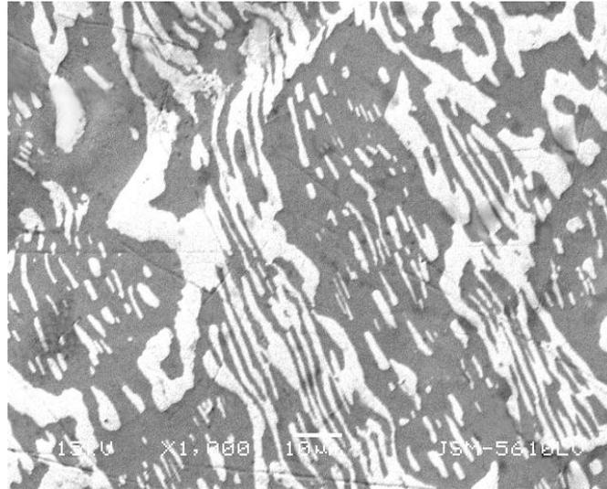
Fig.(e): SEM micrograph for 28.35 At. % Bi and 71.65 At.% Sn
