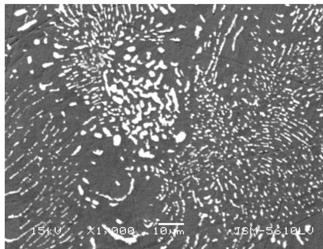
**Fig.(a): SEM micrograph for 7.26 At. % Bi and 92.74 At.% Sn**
