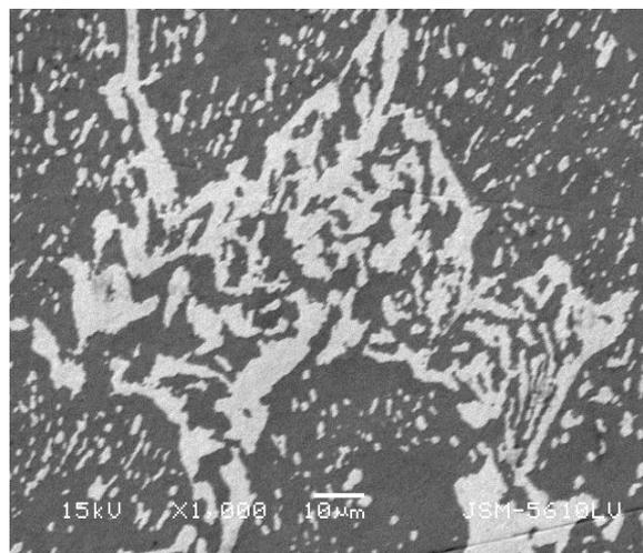
**Fig.(d): SEM micrograph for 26.79 At. % Bi and 73.21 At.% Sn.**
