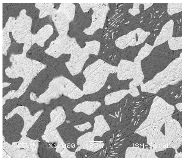
Fig.(g): SEM micrograph for 41.42 At. % Bi and 58.58 At.% Sn
