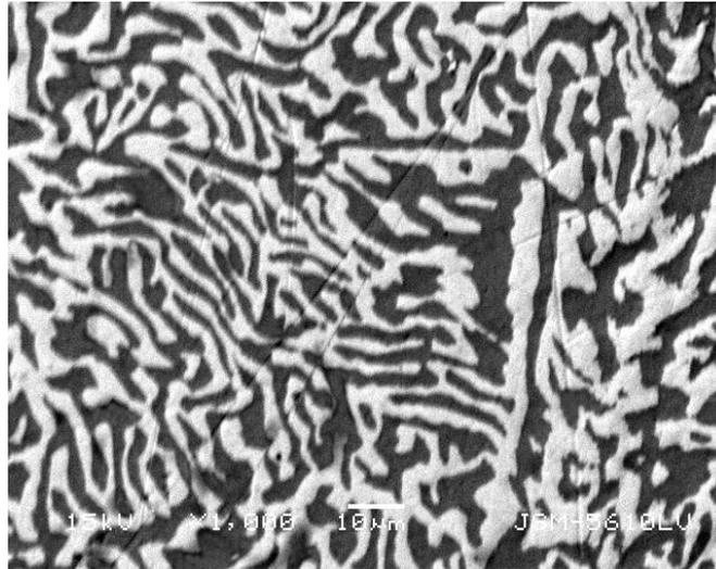
**Fig.(h): SEM micrograph for 47.20 At. % Bi and 52.80 At.% Sn**
