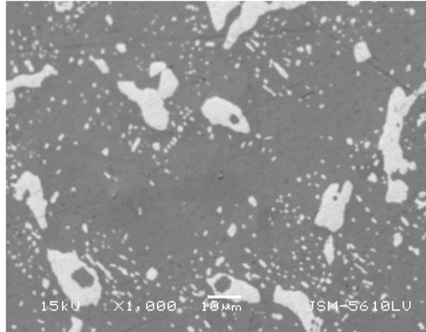
**Fig. (b): SEM micrograph for 12.53 At. % Bi and 87.47 At.% Sn.**
