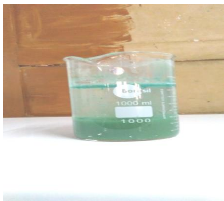
Fig2 Sediment by electrolytic process with copper electrode in Fertilizer Industry Effluent
