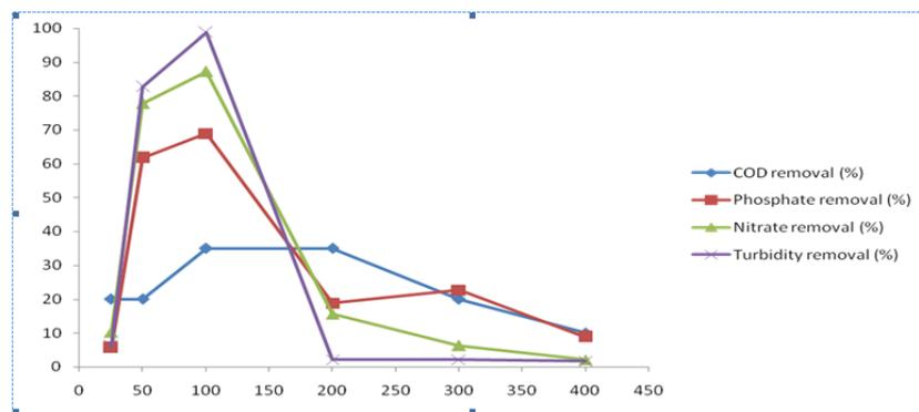
Fig 10 Treatment using FeCl<sub>3</sub> alone at pH= 6
