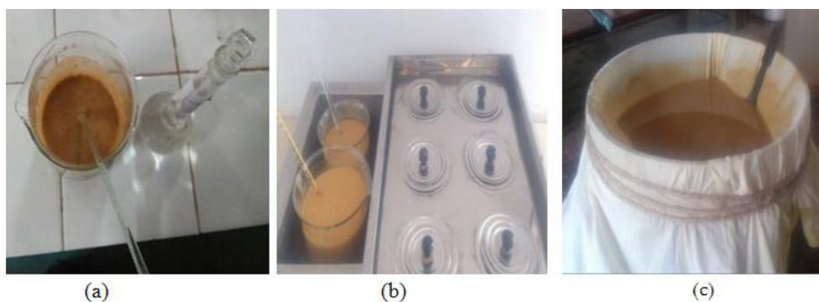
**Fig 2 (a) Peel water mixture (b) Water bath heating (c) Filtration**
