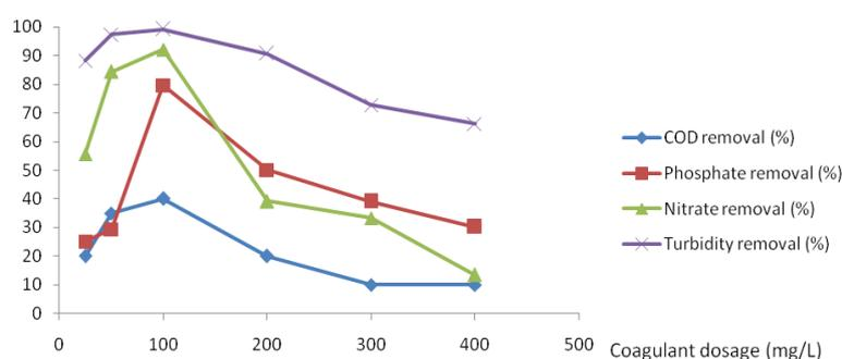
Fig 8 Treatment using  $FeCl_3$  alone at pH= 4
