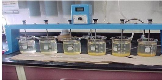
**Fig 4 Conventional jar test apparatus**
