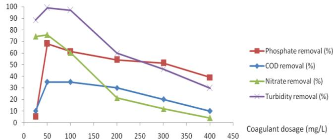
Fig 9 Treatment using FeCl<sub>3</sub> alone at pH= 5
