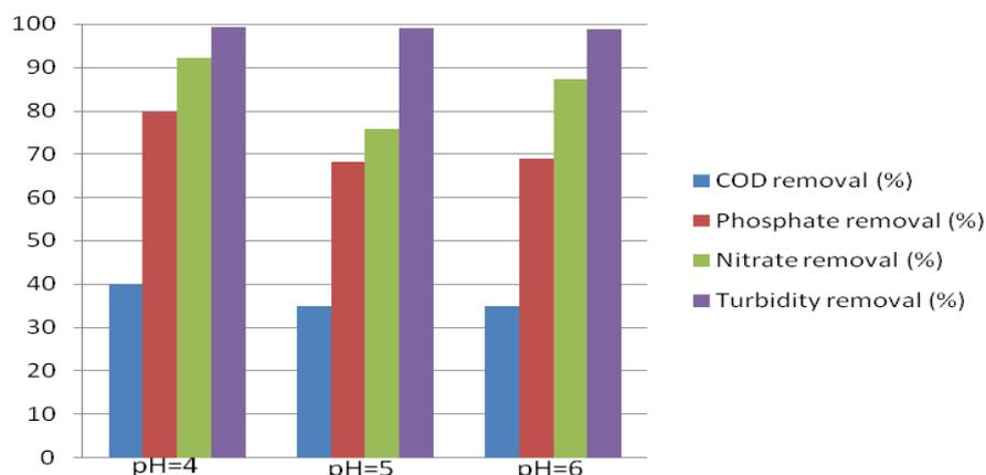
Fig 5.9: Comparison of results at pH=4,5 and 6
