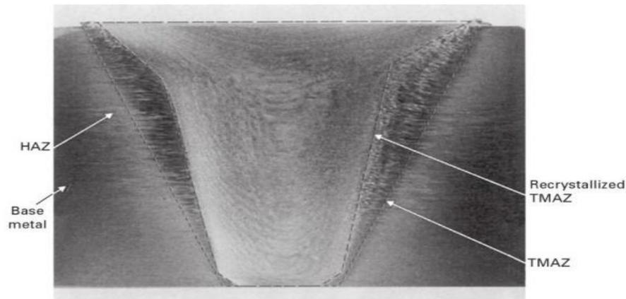
Figure 2: FSW transverse section (Misra & Ma, 2005)
