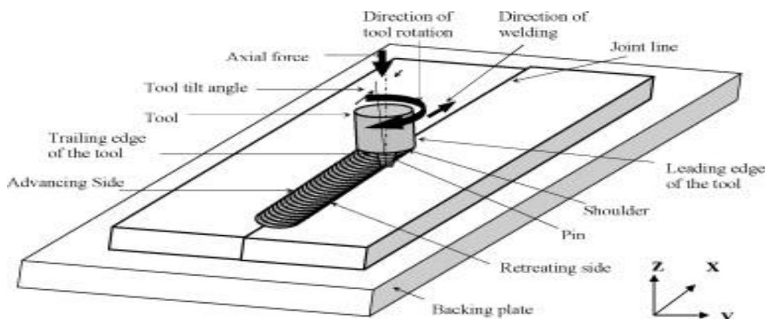
Figure 1: Schematic representations of friction stir welding.[11]
