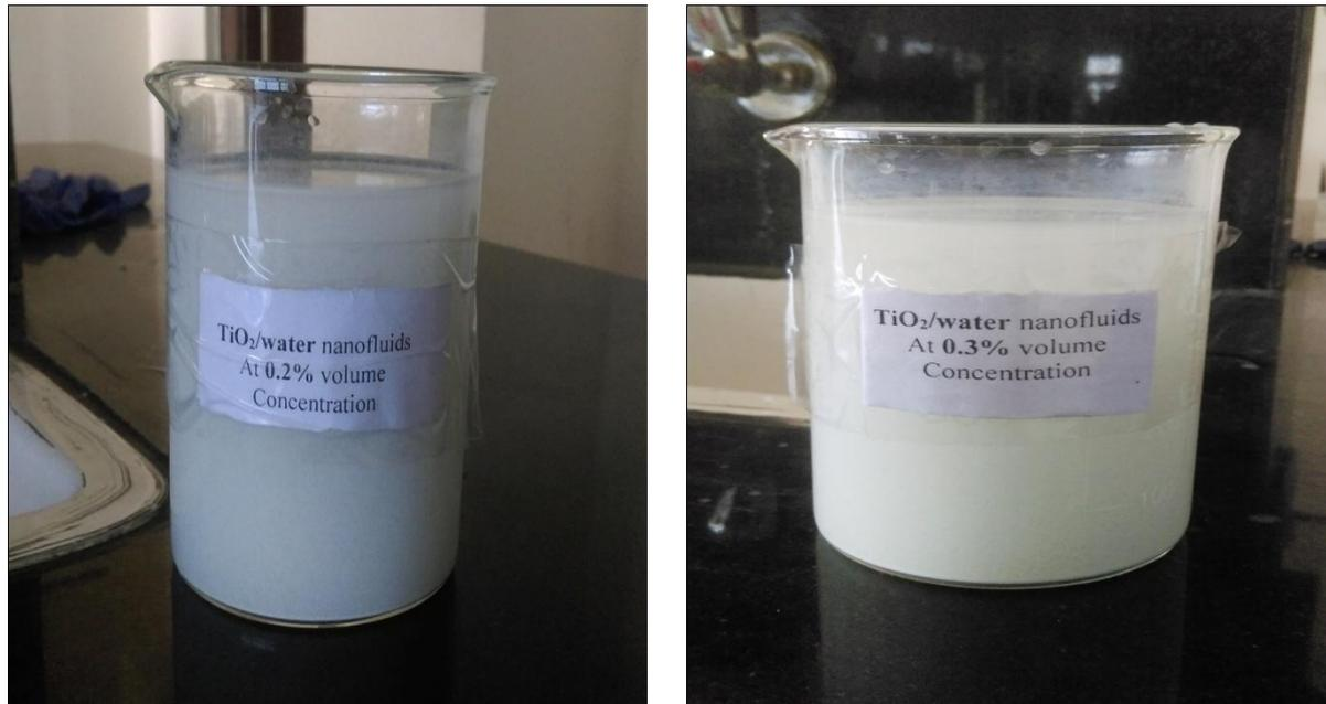
Fig.7: (a) 0.2% concentrations of nanofluids, (b) 0.3% concentrations of nanofluids.
