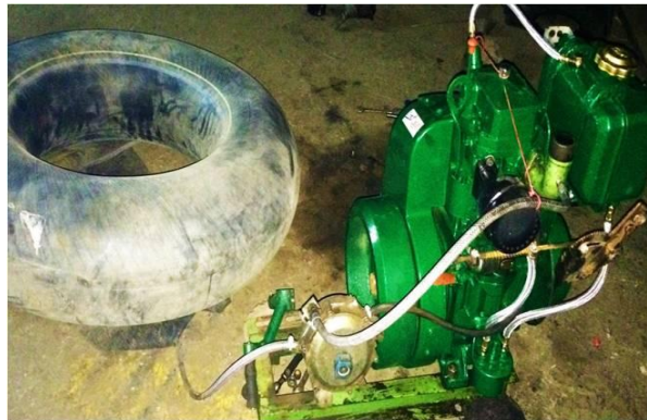
Fig.4 Engine propelled on Upgraded Biogas
