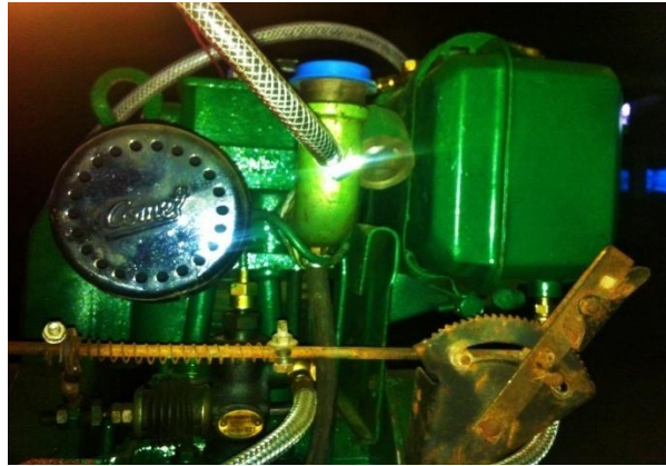
Fig.2 Modified Suction Zone of Engine with Fuel control Ratchet
