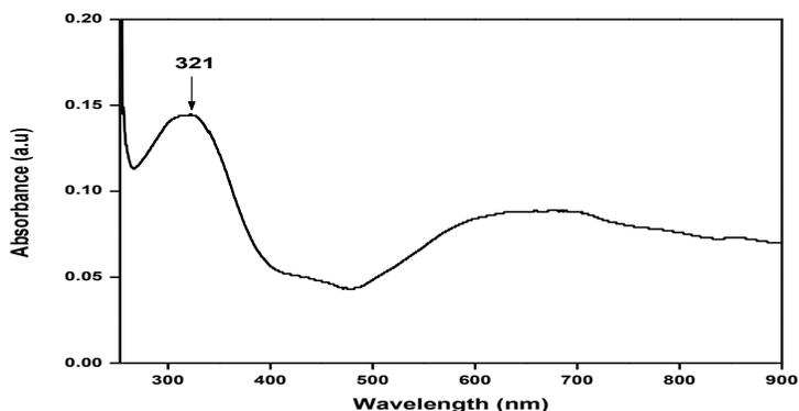
Fig. 4. UV-Vis absorption spectrum of CeO<sub>2</sub> nanoparticles
