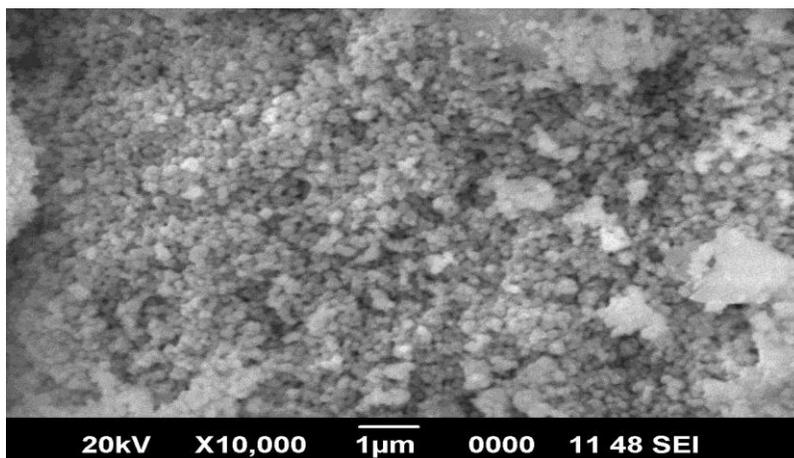
Fig 5. SEM Image of Ceo<sub>2</sub> Nanoparticles
