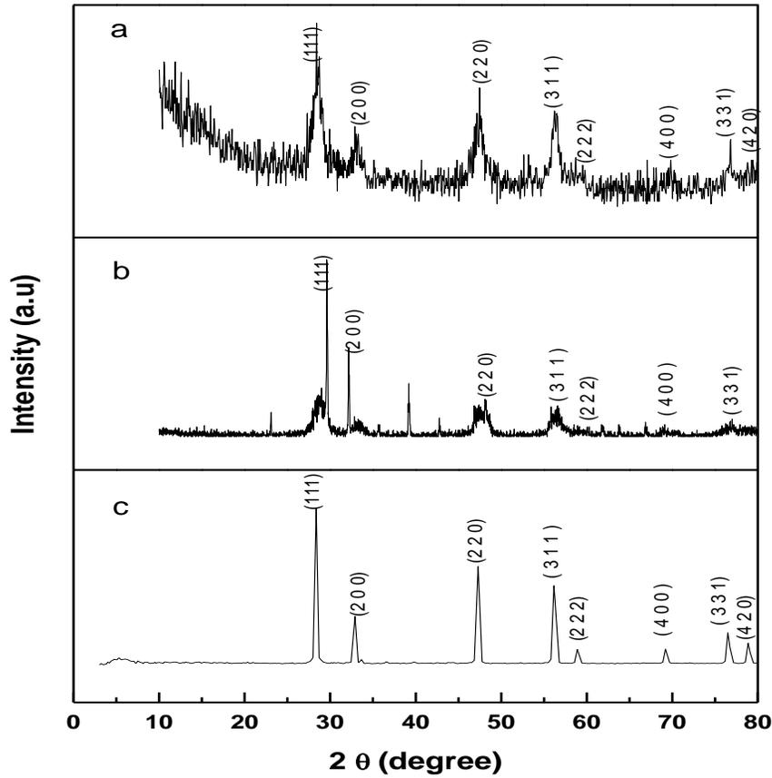
Fig 1. XRD stack view of as-prepared (a) and annealed (b& c) CeO<sub>2</sub> nanoparticles.
