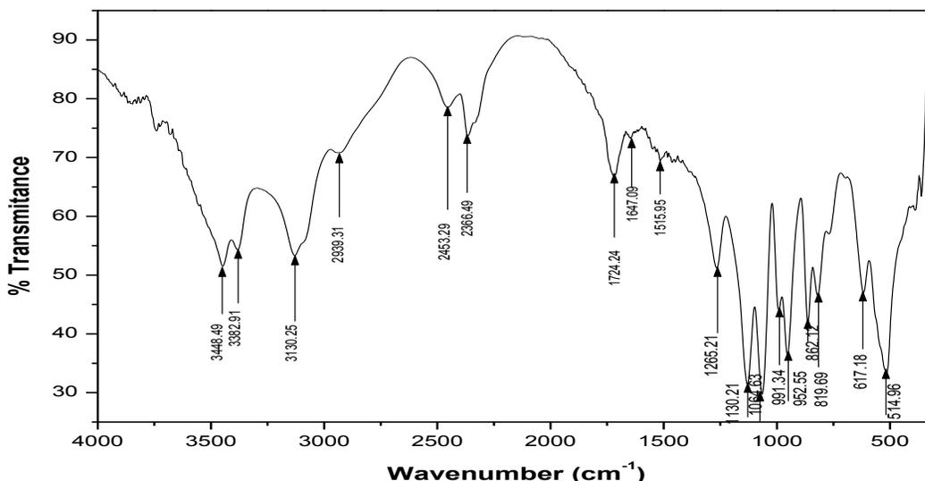
Fig. 3. FT-IR spectrum of CeO<sub>2</sub> nanoparticles
