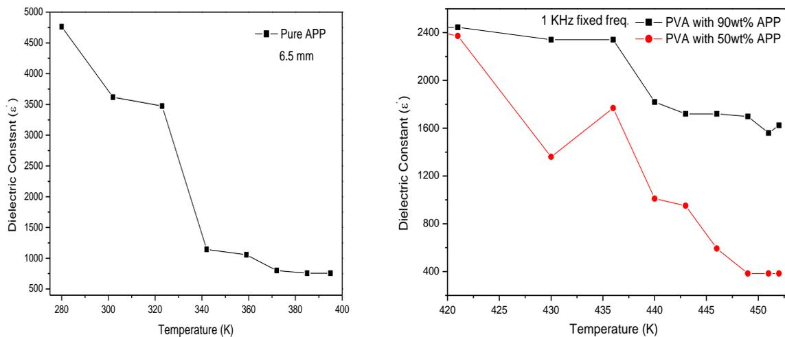
**Fig. 3.2 The APP of Dielectric Constant Versus Different Temperature. Fig. 3.2.1 The Plots of Dielectric Constant Versus Function of at fixed frequency. Temperature for composites of PVA with APP.**
