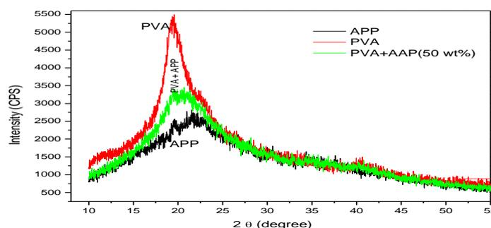
**Fig. 3.1** XRD spectrum for the sample of Pure PVA, APP and PVA with 50 wt % of APP.
