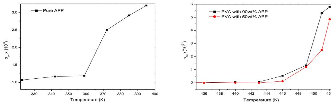
Fig. 3.4 the A C conductivity verses function of temperatures Fig. 3.4.1 The plot of ac conductivity of PVA and its composites with for APP at thickness of 6.5 mm.different weight percent of APP at thickness of 6.35 mm and 3.21 mm.
