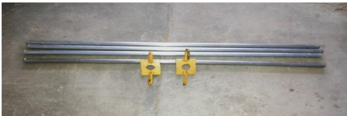
MODEL PILES & PILE CAP
