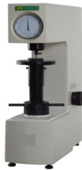
Fig :-Rockwell hardness testing of ball bearing
