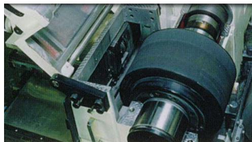
Fig:-centre less grinding
