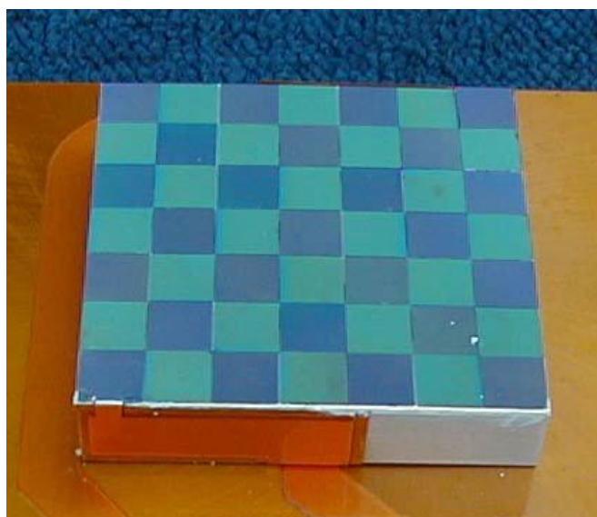
Figure.8:Amonix Dense Packed Array.
