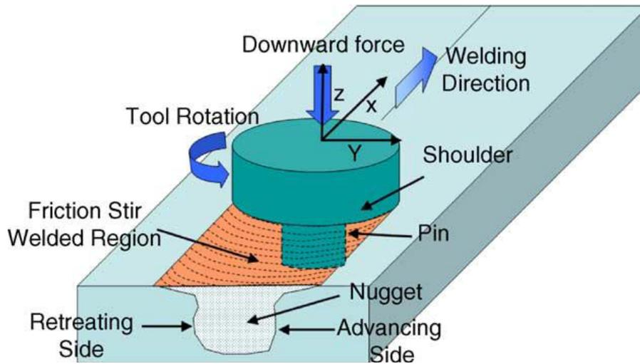
Fig.1 Principle mechanism of friction stir welding [1].
