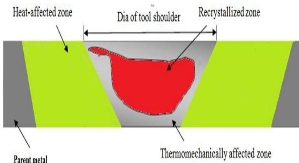
Fig.2 Microstructural regions of friction stir weld.
