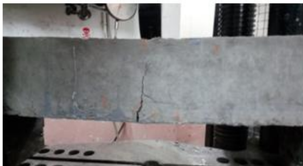
Fig. 13: Failed beam BF4 after testing
