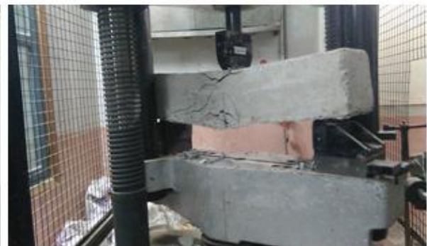
Fig. 12: Failed beam BF3 after testing
