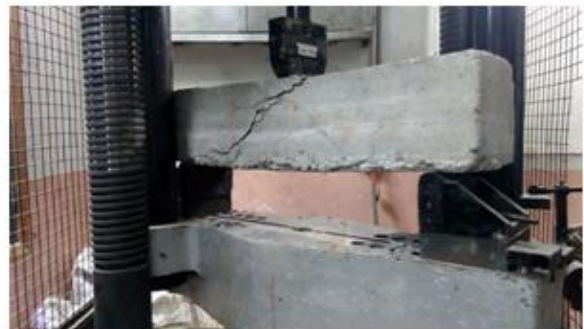
Fig. 4: Failed beam CBS1 after testing
