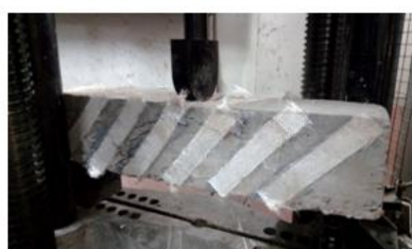
Fig. 6: Failed beam BS3 after testing
