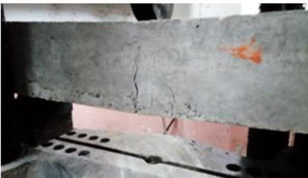
Fig. 11: Failed beam BF2 after testing
