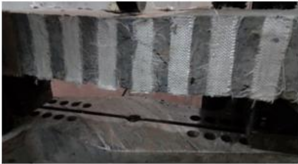
Fig. 7: Failed beam BS4 after testing
