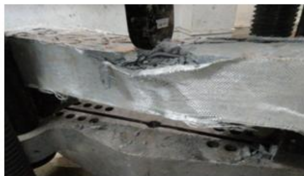
Fig. 5: Failed beam BS2 after testing
