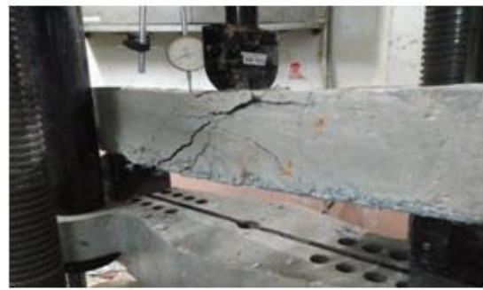
Fig. 2: Failed beam F1 after testing
