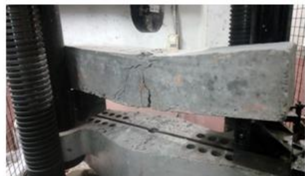
Fig. 10: Failed beam CBF1 after testing
