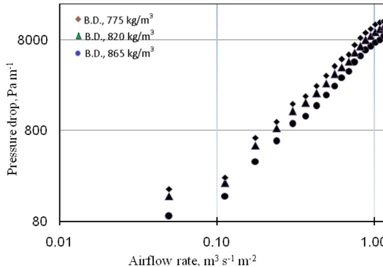
**Figure2: Effect of Bulk Density on Minimum Fluidization Velocity of Lathyrus at Moisture Content Of 13.60% D.B.**
