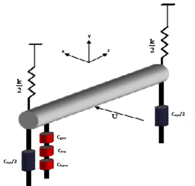
Fig. 6: Simple schematic of a VIVACE module with coordinate system [2].
