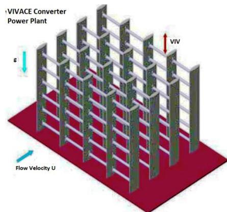
Fig. 7: Small VIVACE converter power plant.
