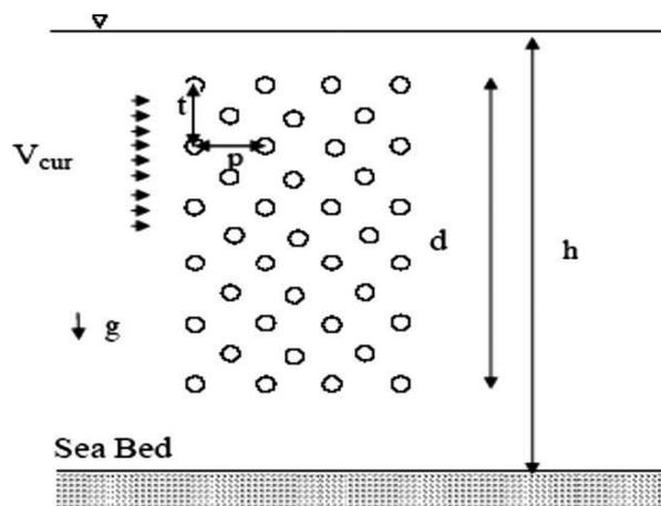
Fig. 8: Geometry, dimensions, and arrangement of cylinders in a VIVACE converter assembly [2].
