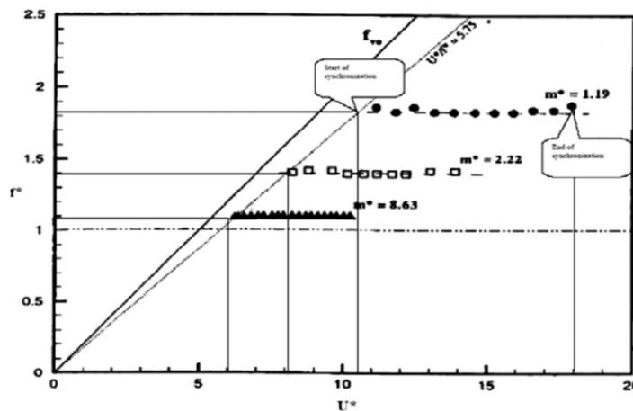
Fig. 4. Lower branch frequency response for different mass ratios versus varying  $U^*$ ; here  $f^* = f_{cyl} / f_{n,fluid}$  [1].
