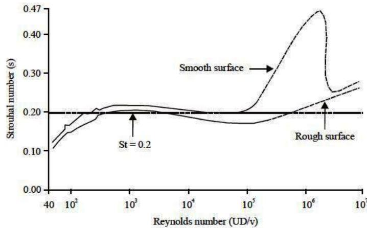
Fig. 3: Curve showing the relationship between Strouhal number and Reynolds number [6].
