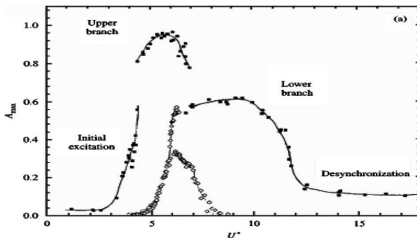
Fig. 5: Amplitude of oscillation Feng’s case, for experiments in air by Feng and experiments in water by Khalak and Williamson [11].
