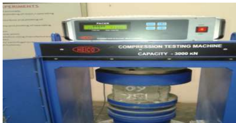
Fig. 1 Compression testing of sample in digital compression testing machine
