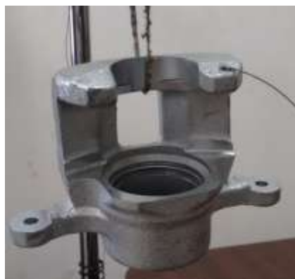
Fig.2 Accelerometer location on caliper with free hanging condition
