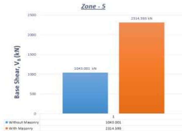
Figure 5 Base Shear Comparison Graph for zone-5 building with/without masonry
