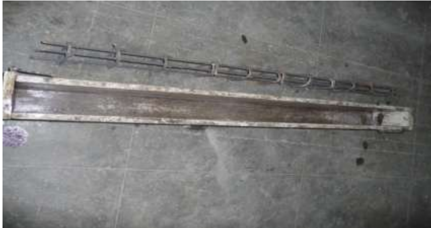
Fig.1. Mould and Reinforcement Cage for Casting MRFC Prototype beams.
