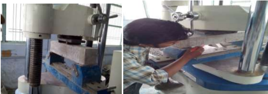
Fig 8: The method of loading used was Two Point Loading system
