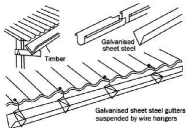
**Fig 1: Guttering materials**
