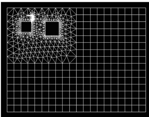
Figure 3. Finite Element Mesh of Crack at Corner of Cut-Out
