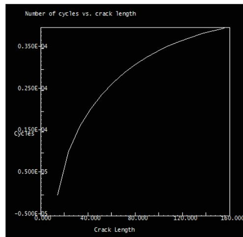
Figure 6. Crack length Vs No. of Cycles plot of Steel Plate with Rectangular Cut-Outs 300 mm apart
