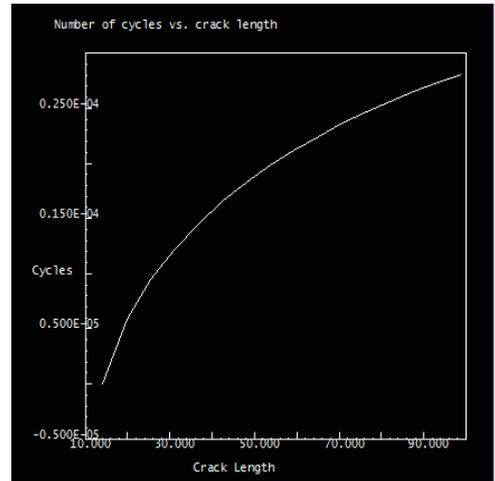
Figure 8. Crack length Vs No. of Cycles plot of Steel Plate with Rectangular Cut-Outs 500 mm apart
