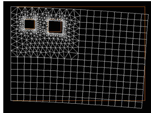
Figure 2. Finite Element Mesh of Deformed Shape of Steel Plate
