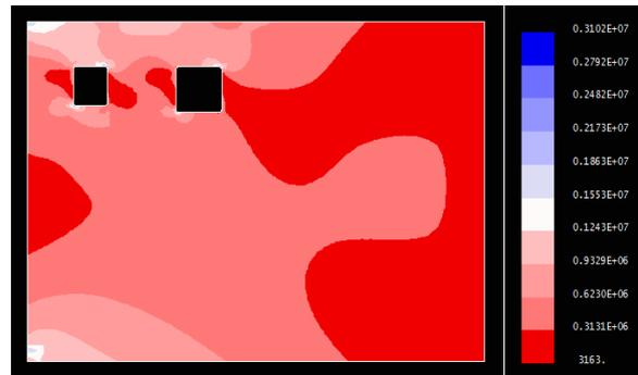
Figure 10. Von Mises Stress Plot of Steel Plate with Rectangular Cut-Outs 300 mm apart
