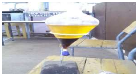
Fig. 2 shows separation of glycerol from Jatropha methyl ester in a separating funnel.
