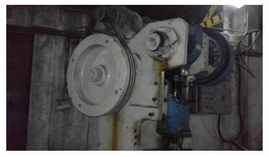
Fig 1. Actual Flywheel Given data, Motor specifications:-8HP Motor & Revolution1000 RPM,
