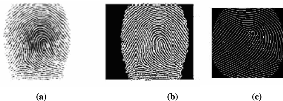
Figure 7: a) Original Image b) Binary Image c) Thinned Image
