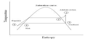
1-2 Heat applied to evaporator through external sources vaporizes working fluid to a saturated (2') or superheated (2) vapor.
