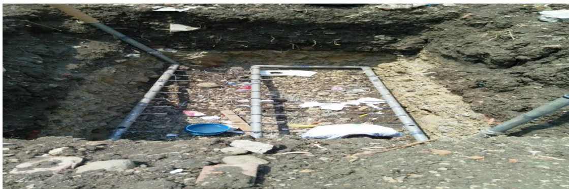
Fig 6 Experimental setup of series connection (2.5 m) without covered soil with fins
