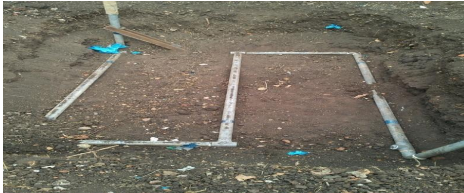
Fig. 5 Experimental setup of series connection (2.5 m) without covered soil
