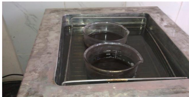
Figure 3: Ultrasonic Cleaner apparatus for sonication process of CuO Nanofluids
