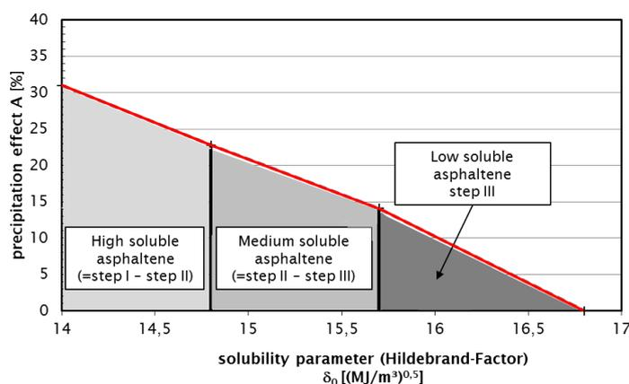
**Figure 2: Explanation to Three Asphaltene Fractions in Bitumen**
