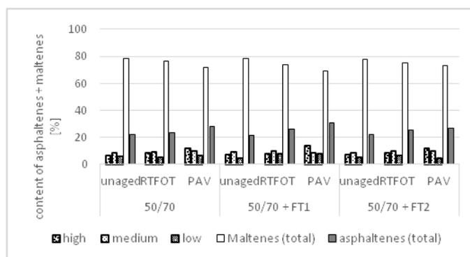
**Figure 9: Content of low, medium, high soluble asphaltenes, total asphaltenes and total maltene content**
