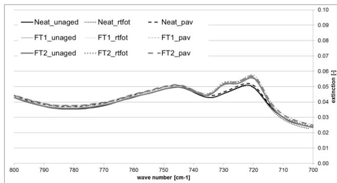
Figure 15: Identifying Wax Modifiers in Bitumen
