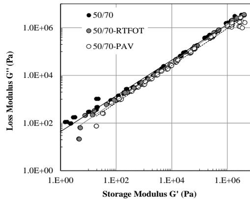
Figure 5: Cole-Cole-plot of the DSR-temperature-frequency sweep tests obtained on the unaged, short- and long-term aged samples of the straight bitumen 50/70 – addition of fitting curves
