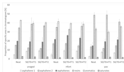
Figure 7: SARA components of unaged and aged binders
