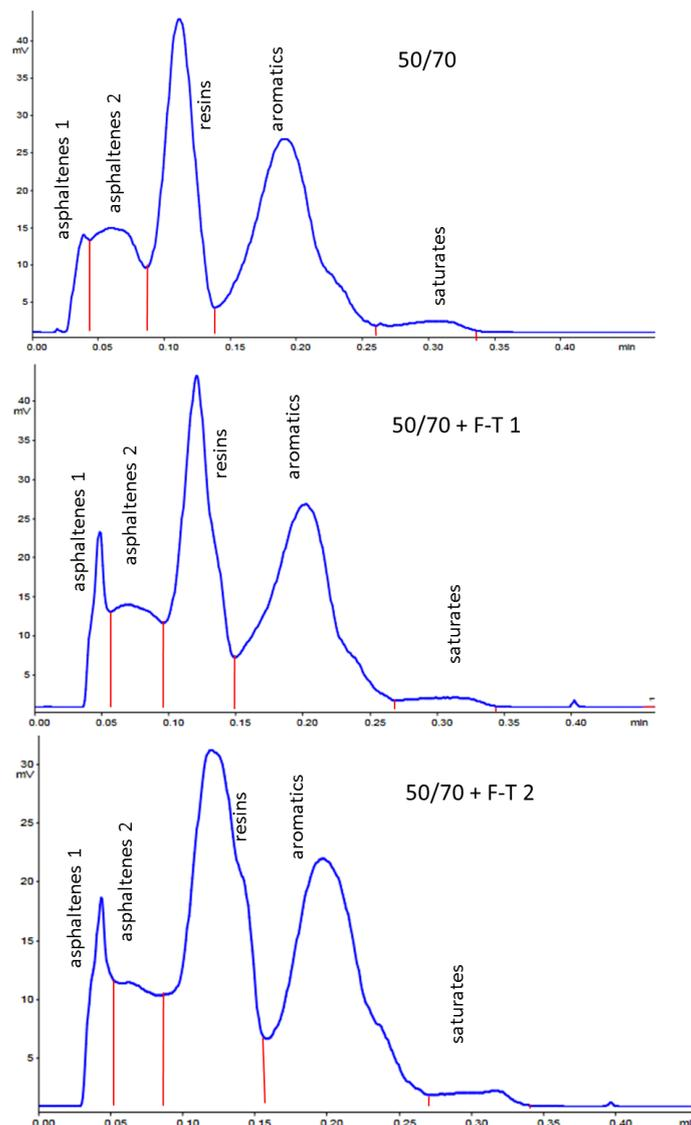
Figure 1: Chromatogram for SARA Components of 50/70 (unmodified and Modified)
