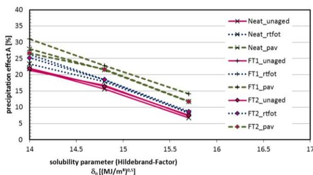
**Figure 10: Profile of solubility and precipitation limits**
