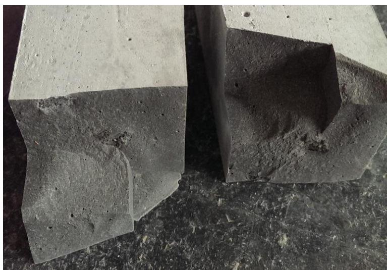
Figure 5: Non-standard fracture plane after three-point bending test
