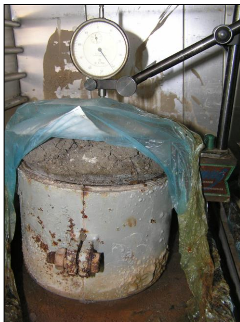
Figure 10: View of a sample compacted by 100% Standard Proctor energy at the temperature of 75°C after 65 days
