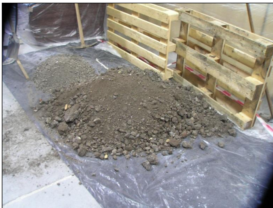
Figure 2: The steelwork waste (heap on the right) with debris of metallurgical ceramics excavated from the pit under the floor of the Demos hall in Ostrava (11/2014)
