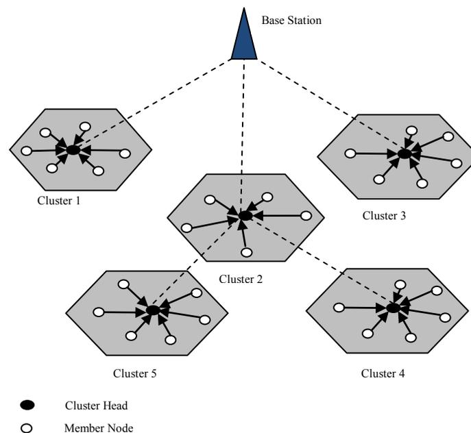
**Fig. 2 Multihop Communication for Larger Network in M-LEACH**
