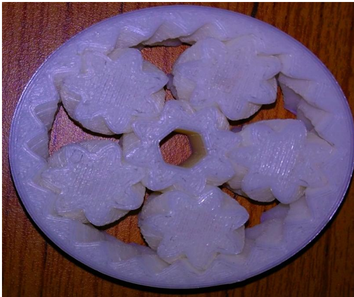
Fig: 3D Print of sun and planetary gear
