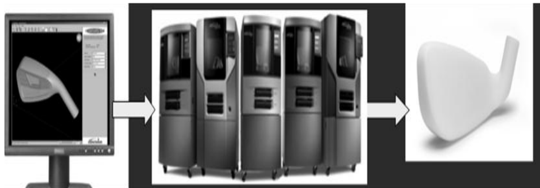
Fig 1.14. General principle of 3D printing
