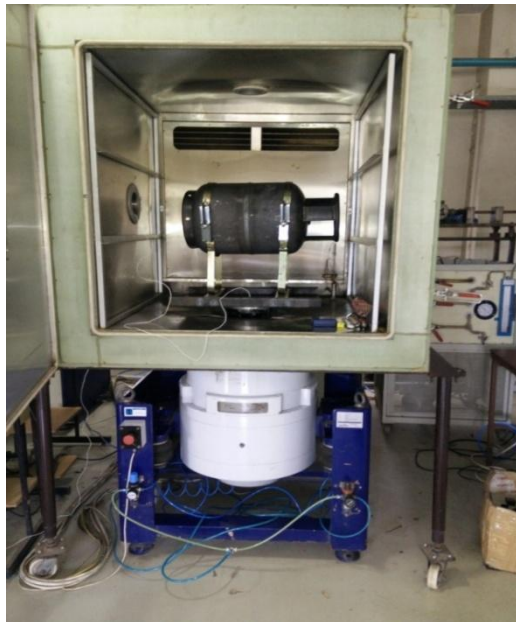
Figure 5: LPG cylinder mounted for vibration test on shaker table.
