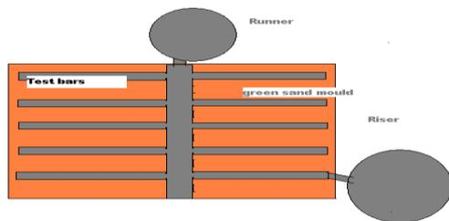
Figure 1(a). Sample casting green sand mould
