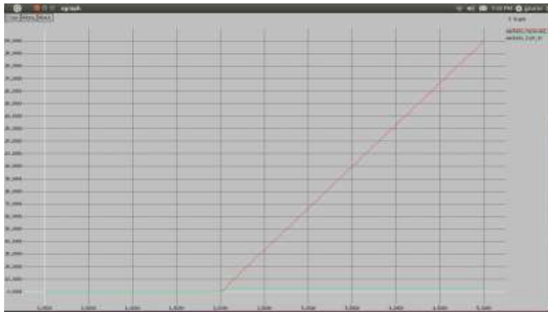
Figure 3.7: Graphical Representation of Transfer of Packets for 50 Nodes with One Node as Wormhole
