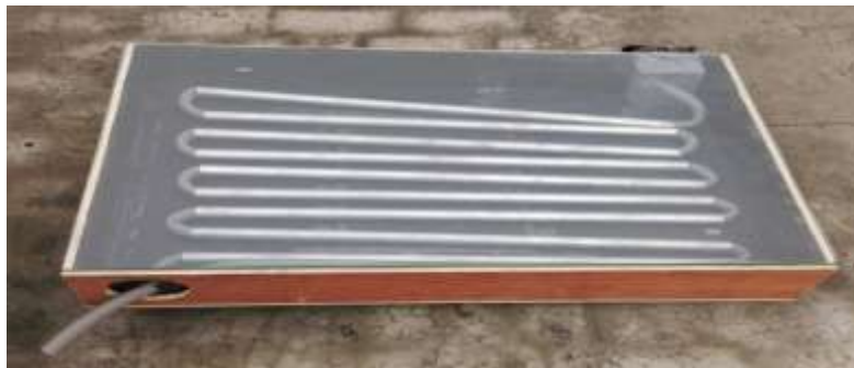
Figure 1. Solar Air Collector
